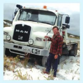
truck has a massive tilt tray and slide and a 6 ton winch. It runs on 10.00 x 20 tubed tyres and carries 560 litres of diesel when fully fuelled up. It has a 10 speed road ranger crash gear box and a rear diff lock, and it's a veritable tank of a vehicle.
